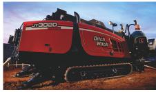
tively affecting other functions. Built up from the JT2720, the self-contained JT3020 provides 30,000 pounds of pullback and the capacity to bore pilot hole diameters up to 4.5 inches and backream diameters up to 12 inches. Meanwhile, the sound level is less than 82 dB(A) at the operator's ear. A redesigned machine anchor system is easy to set up and holds firm in various soil conditions. Estimated list price: \$215,000 to \$275,000.
