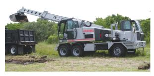
predecessor did. This conserves fuel, the company says, while producing greater horse-power and operating both the truck carrier and the upperstructure. Upper-structure swing speed has increased 33 percent, and breakout force increased from 21,900 to 24,900 pounds. New electronic joysticks replace hydraulic controls, and three joystick patterns are available. Models are offered in 6x4 and 6x6 configurations and can travel on highways at 55 mph. Estimated list price: \$320,500 to \$340,000.
