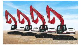
that provides up to 10 percent more hydraulic horsepower. Two-speed boom lifting and arm open/close functions work with hydraulic-system regeneration for faster cycle times, the company says. The series includes Link-Belt 160 X2, 210 X2, 240 X2, and 290 X2 — ranging in operating weight from 37,700 to 65,700 pounds.
