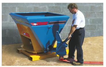
Stone designed Groutzilla to clean up in just a few minutes with no disassembly. But its discharge snout can swing away on heavy-duty hinges for visual inspection as necessary.
