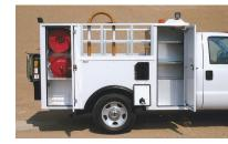
long. It can carry up to 10 truck tires. An air compressor is included, covered by a heavy-duty bulkhead that protects it from the elements and shifting loads.
