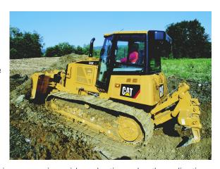
control of each track for precise maneuvering, quick acceleration, and on-the-go direction changes. Its undercarriage has an oscillating track roller frame, which is said to keep more of the track on the ground in uneven terrain. It is powered by a 125-flywheel-horsepower Cat C6.6 engine, which is 5 dB(A) quieter. Estimated list price: \$200,000.
