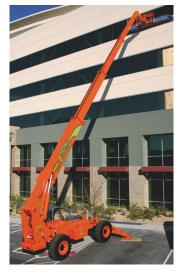
(rated at 49 gpm and 4,000 psi) and a quick-attach system. Among a selection of optional work tools are a utility bucket, concrete bucket, truss boom and wallboard/sheet material handler.
